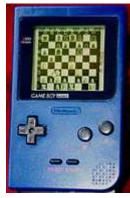
Overall, the GameBoy Pocket unit, pictured here measures 5 inches long by 3 inches wide. The thickness of the GameBoy Pocket unit is nearly 1 inch. The GameBoy screen has a diagonal measurement of just over 2.5 inches. (Screen dimensions are 1 15/16" wide by 1 3/4" high). Interestingly enough, the GameBoy
