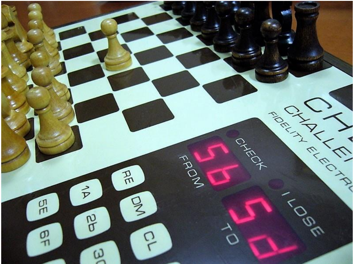
Chess Challenger 1 has a clearly readable display! White plays 5b-5d, which means pawn from e2 to e4.
