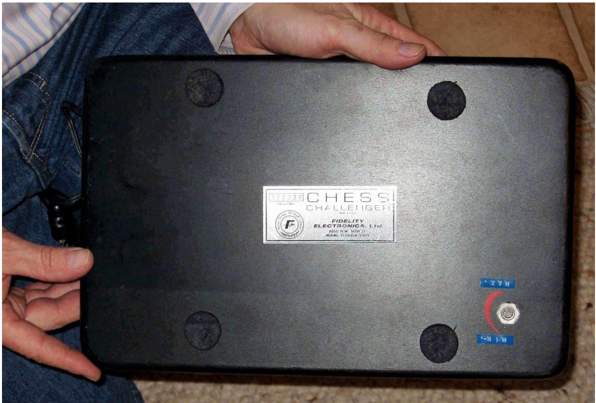
Luuk's Voice Chess Challenger with the adjusting screw to temper the voice!
