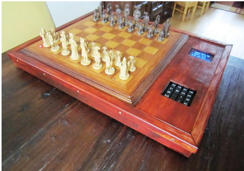
Chess computer with program WChess Own construction by John Dijkstra (Deventer - the Netherlands)
