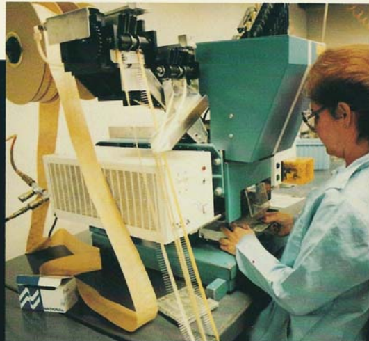
Automatic Insertion—Resistors and Diodes.
