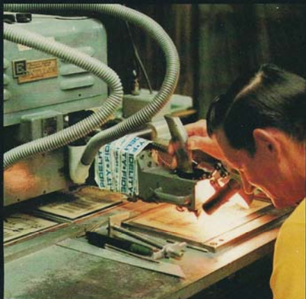
Printed Circuit Board Drilling Machine.
