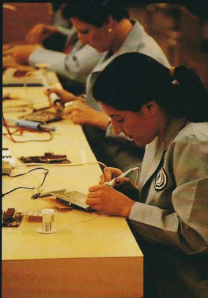
Precision Hand Soldering.
