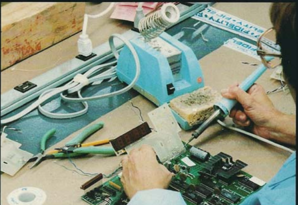
Hand Soldering—Display to Printed Circuit Board.
