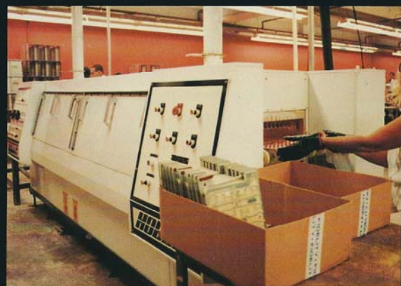
Automatic Printed Circuit Board Cleaning Machine.
