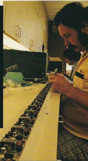
Production Electronic Circuitry Environmental Control System.
