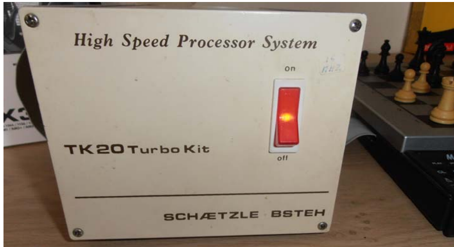
High Speed Processor System - TK20 Turbo-Kit (16 MHz) with Ed Schröder's Experimental MM V Program (foto: Hans van Mierlo - 21.01.2013)
